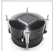
The EKL 22201 consists of an extrusion profile and dissipates the heat from your processor ideally and reliably. With a compact height of only 60mm, this cooler is ideal for all compact PC systems, workstations or even for the normal office PC. The built-in fan has a 4-pin connection and can therefore be controlled manually via the mainboard. This enables an adjustable speed range of 500-1800 rpm. Thanks to the PWM signal, the fan operates depending on the workload of the CPU.
