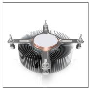
With an extremely low height of only 30mm, the EKL 22205 is ideal for compact PC systems in the small form factor area. Especially in this size range it is often difficult to get a powerful and at the same time quiet CPU cooler. The EKL 22205 masters both challenges. The interaction of an aluminum profile with a copper core, high-performance thermal paste and a low-vibration PWM-controlled fan guarantees quiet and extremely effective heat dissipation.
