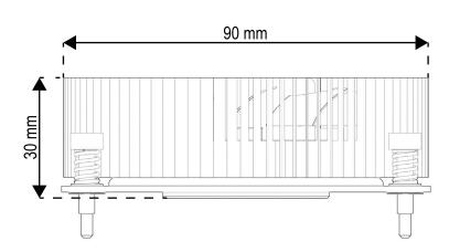
The thermal and mechanical compatibility can vary depending on the system used. All information according to manufacturer specifications. The maximum tightening torque for screw mounting is 1 Nm. Data subject to change (02/23).
