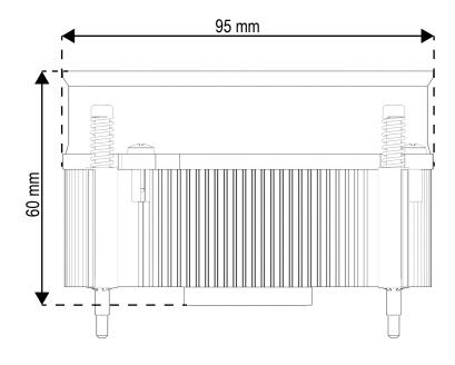
The thermal and mechanical compatibility can vary depending on the system used. All information according to manufacturer specifications. The maximum tightening torque for screw mounting is 1 Nm. Data subject to change (11/21)
